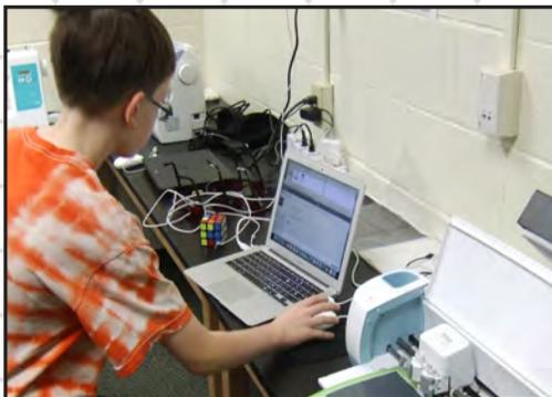
*Daniel uses the Cricut Design Space to create an image to send to the die cut machine and create a vinyl decal.*
